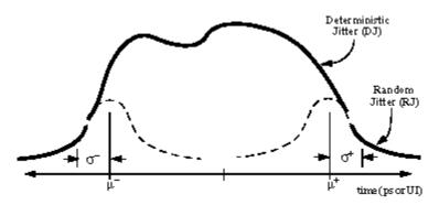
First, the tail region of the histogram of measurements for a given pattern span is isolated. Then, an optimization routine is used to determine the best-fit coefficients from which the 1-sigma value is obtained. This operation is performed on three or more pattern spans to ensure reasonable frequency coverage from the corner frequency to Nyquist. The number of pattern spans selected will affect the acquisition time and can be adjusted using the *Tail-fit* option.
